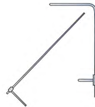
Figure 2: Straight Pitot and Standard Pitot Tubes.
