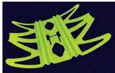
The saddle measures 12 x 14 x 2.5 and is installed on the existing strapping to straighten flexible ducts and improve airflow.
