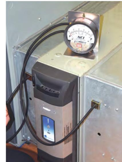
Measuring air filter pressure drop.
