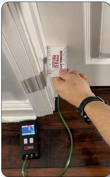
Measuring room static pressure with a "Roomulator" and a micromanometer.
