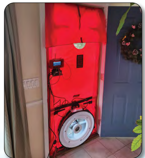
Blower-door instrument seals outside door for pressure testing the building and find leaks.
