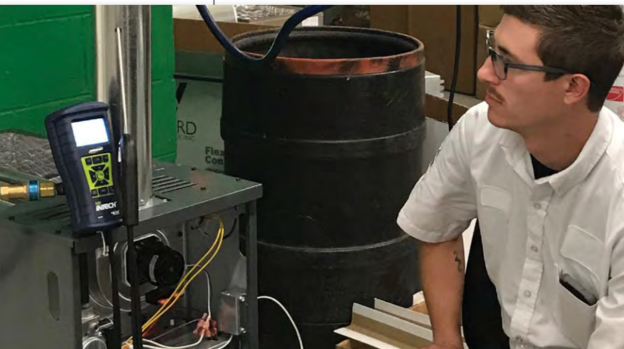
Combustion analyzers are key instruments for testing and diagnosing issues that can lead to CO production.
