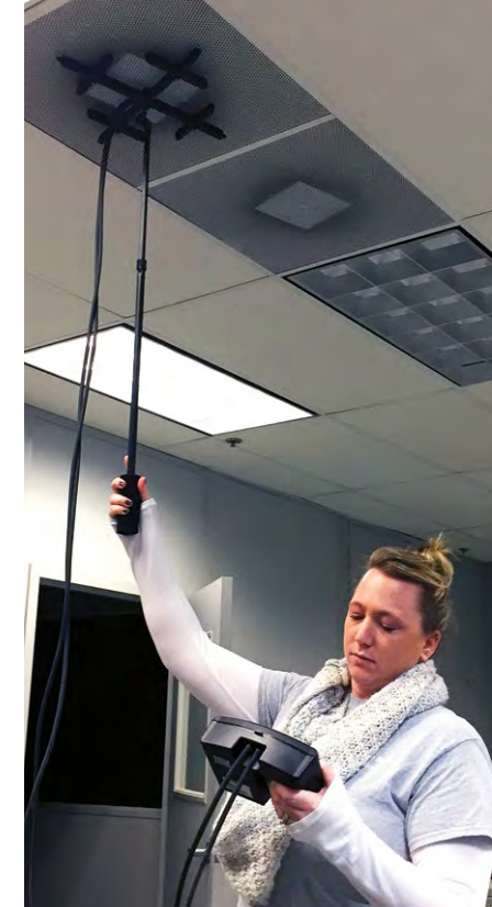
Dawn Vickers-Mroczek of GVs Heating and Cooling, Glenview, IL uses a VelGrid.
