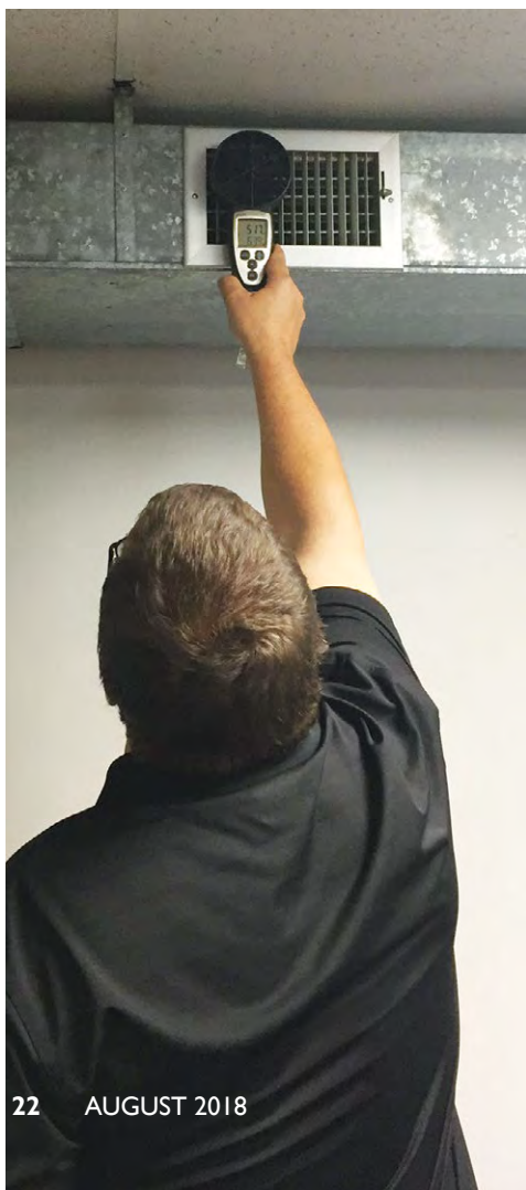
Joseph Kosky of the University of Pittsburgh, using the Rotating Vane Anemometer.
