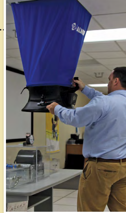
Airflow measurements with flow hoods are a key component of NCI's High-Performance training.
