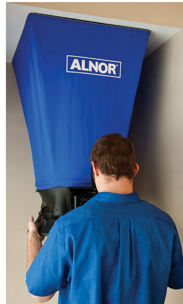
Using a flowhood, HVAC technicians can accurately measure airflow at the grille.
