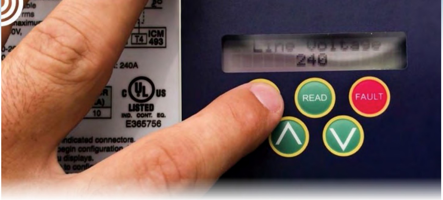
There is a steady-state voltage problem that can take out inverter boards. Inverter-driven equipment refers to a variable-frequency drive with ECM compressors and fans that can be damaged by power outages. Image courtesy of HVAC School.
