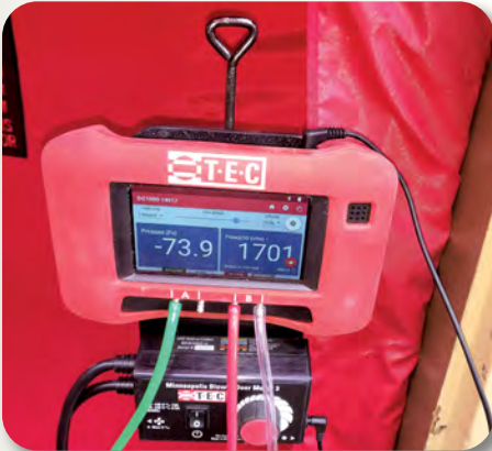
A-Team checked the pressures inside the home using a blower door test.
