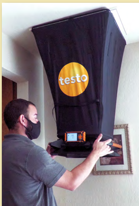
Using a balancing hood helps to make air visible in each room of a home. Bailey Heating and Air uses these instruments to test airflow before and after they work on a system.
