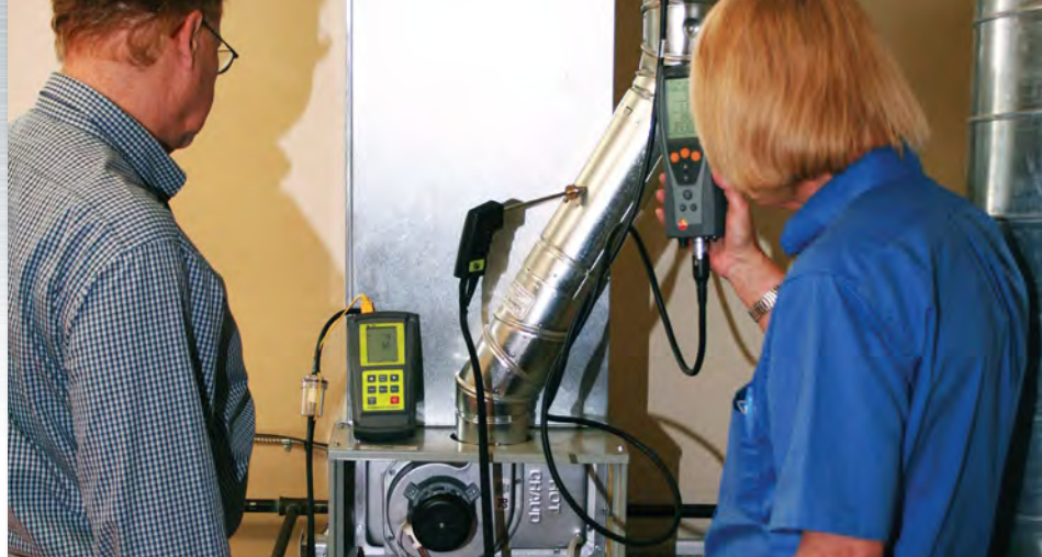
Jim Davis (right) demonstrates how to use a combustion analyzer to determine whether flue gases are "sick" or not on a live furnace.
