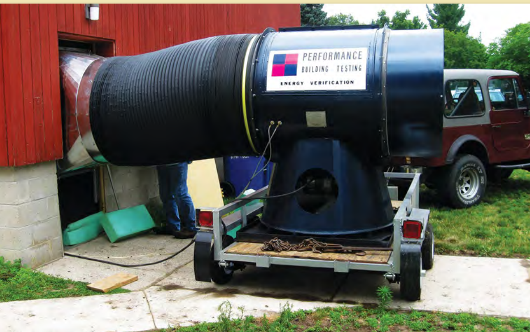
Integrity Test and Balance, Inc. sets up to do a building performance test on a church facility.
