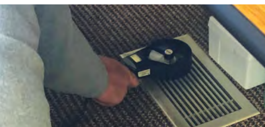
Using a vane anemometer, this technician measures air velocity, volume flow, and temperature as well as airflow at registers.
