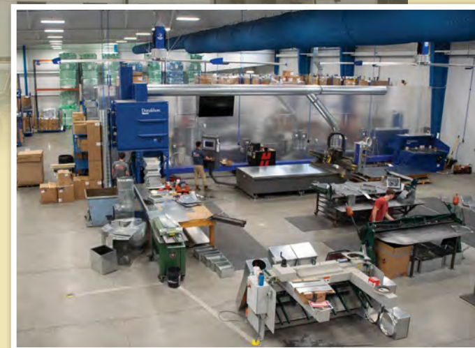
A bird’s-eye view of the sheet metal fabrication shop and the state-of-the-art dust collection system.
