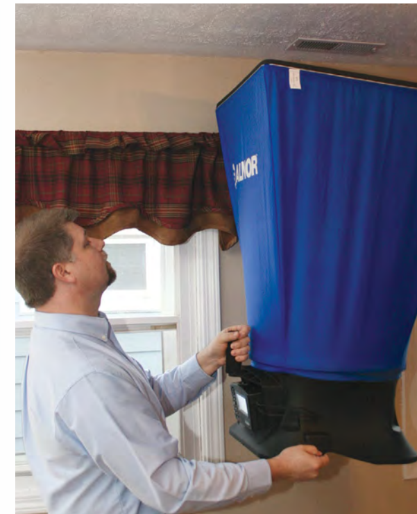
David Richardson demonstrating how to use an air balancing hood to measure airflow.
