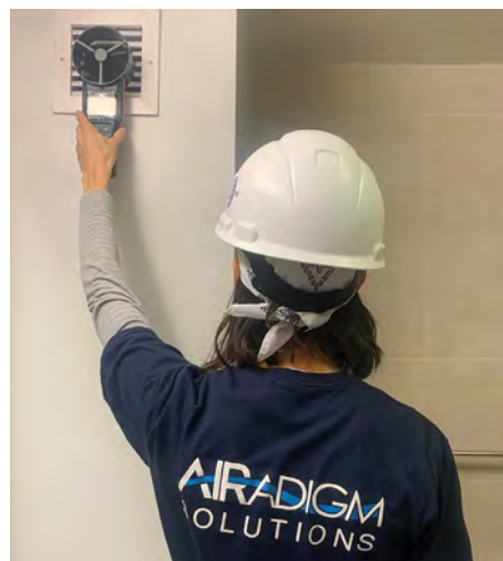
An Airadigm Solutions technician uses an RVA to measure a sidewall grille. Using an RVA on this type of grille will give you the most accurate reading.
