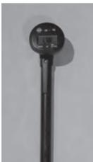
A digital hygrometer is very handy for measuring wet bulb temperatures. As you learn to test enthalpy change when calculating CSER™ you'll find accurate wet bulb measurements are critical. Digital hygrometers typically range from \$100 to \$200.
