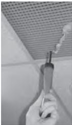
Titanium Tetrachloride puffers produce a realistic smoke that stays visible and buoyant for a long time making it easier to trace air patterns, find leaks, etc. The downside is the chemical is highly corrosive and toxic and should be used sparingly. Be careful not to place in contact with eyes or breathing in the smoke. Keep them in an airtight container as the corrosive chemical is very harmful to electronic instruments.
