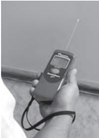
An infrared thermometer is a must-have tool for diagnosing system performance. It can be used for a variety of diagnostics tests including measuring grille temperatures, calculating wall and ceiling R-values, finding missing insulation, identifying thermal bypasses, and more.
