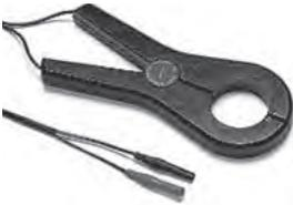
When adjusting pulleys to increase airflow on belt driven blowers, it's critical to check amp draw so as not to overload the motor. In order to get accurate airflows and amp draw, this must be done with the blower compartment door on. A one-piece clamp-on meter won't work in this scenario. A clamp with a 3 ft. lead is needed to perform the test. Remote clamps come as plug-ins or standalone units ranging from \$100 to \$300. Fluke makes several models that will do the job.
