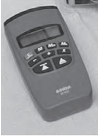
While you can measure rooms with a tape measure to calculate heating and cooling loads, this device, typically available with a laser target for less than \$100, speeds up the process and helps you project a more professional image with your customers. They take practice to get reliable numbers, but allow quick, reliable room measurement.
