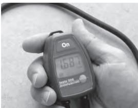
High quality digital manometers have recently come on the scene. Some are extremely accurate, have multiple pressure ranges and are very durable. Digital gauges do not need leveling – a
