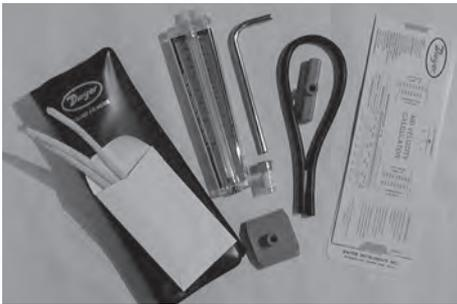
Draft gauges are important instruments for troubleshooting combustion systems. While there are digital gauges available, an inexpensive, extremely durable Dwyer 460 Air Meter does the best
