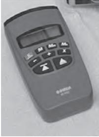
While you can measure rooms with a tape measure to calculate heating and cooling loads, this device, typically available with a laser target for less than \$100, speeds up the process and helps you project a more professional image with your customers. They take practice to get reliable numbers, but allow quick, reliable room measurement.
